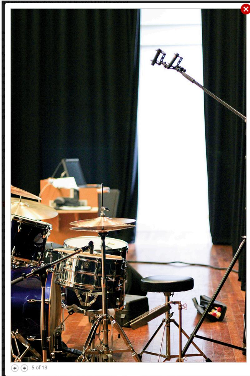
The drum overheads were originally placed behind the drum kit, but spill from the brass sections led us to move them, so that they pointed towards Myles from the front of the kit.
